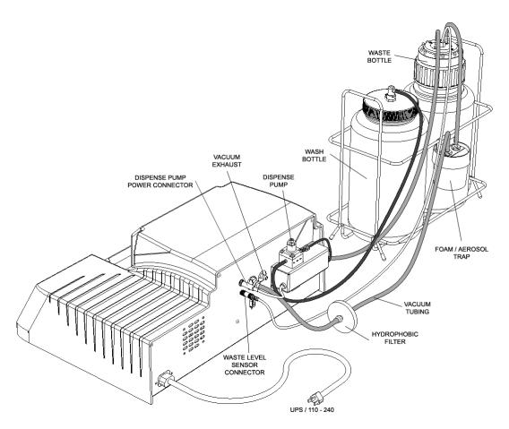
Figure 3. Rear View of the *Opsys* MW™ System
